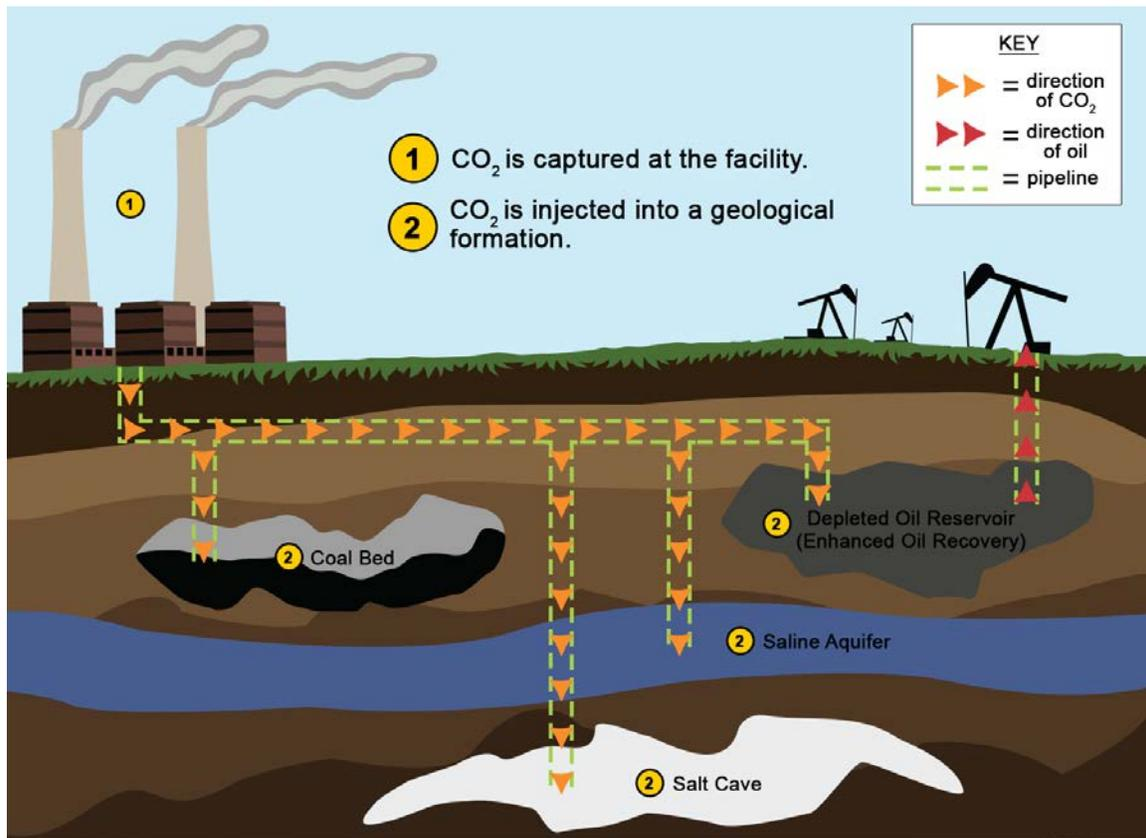
**As global emission requirements for carbon dioxide (CO<sub>2</sub>) continue to become more stringent, existing and new thermal power projects may look towards CO<sub>2</sub> capture, utilization, and storage to remain viable and emission compliant.**
