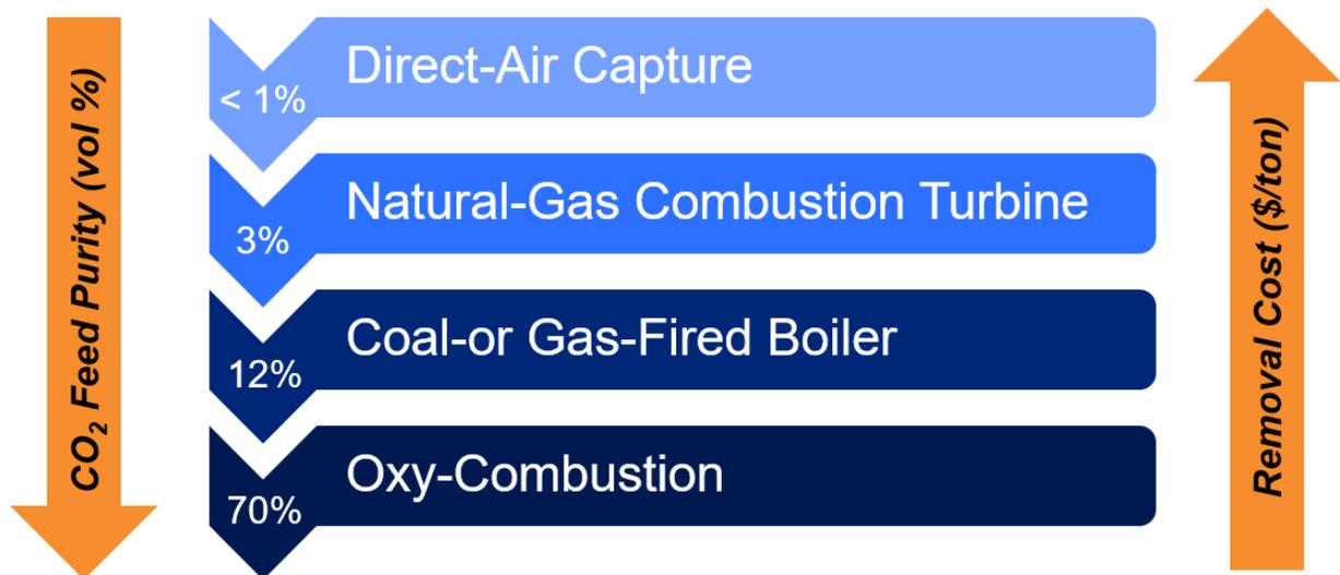
For natural gas turbine applications, the cost of CO<sub>2</sub> capture is much higher than coal-fired boilers due primarily to the low CO<sub>2</sub> density in the flue gas (3% versus 12%). Natural gas applications would typically range between \$60 and \$90 per tonne.
